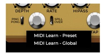
**MIDI Learn - Preset**: this will store the MIDI bindings at Preset level. Preset level bindings have priority over Global Bindings, meaning that assigning a MIDI PC or CC message at Preset level will override existing bindings of the same messages at Global level, if any.
