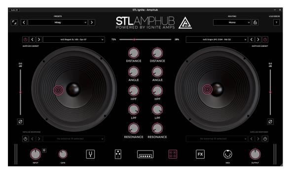
In addition to moving the microphone around the speaker, you can further tweak your tone by using the featured Hi/Lo pass filters and Resonance control, change the volume of each microphone by using the related volume slider, flip the phase with the related button and set the mix of the 2 to find the perfect balance.
